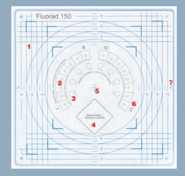
The overall size of the test body for the FLURORAD 150 is 300 mm x 300 mm x 18,5 mm. The copper plate within the details is embedded in acrylglass-plates.
